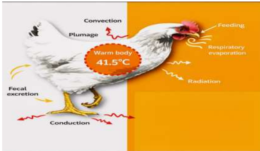
Figure 11: Main modes of heat transfer between the animal and the environment
