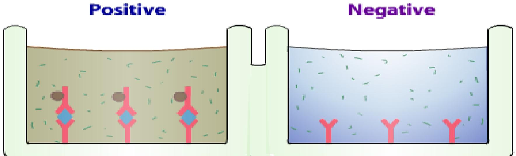
The enzyme's substrate is now added. A color change reveals the presence of enzyme-labeled antibody as well as its bound antigen. No color change indicates that antigen was not present in the test fluid—a negative test result.
