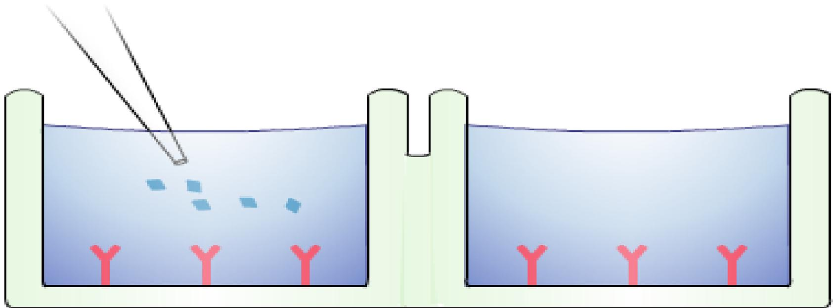
A suspension of serum or other fluid is added to the well to test for the presence of a complementary antigen. In this example, the sample on the left contains the complementary antigen whereas the sample on the right does not.
