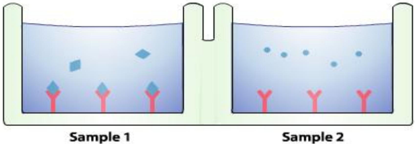
Binding of the antigen to the antibody is strong enough to withstand rinsing that removes the test fluid and unbound antigen.
