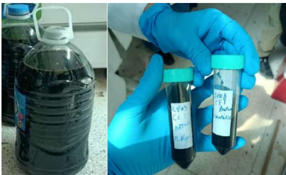
Fig. 13. Leachate sample containers: 5 L bottles for physicochemical analysis (left) and 50 mL tubes for microbiological analysis (right) (Hamiouda & Karaali, 2024).
