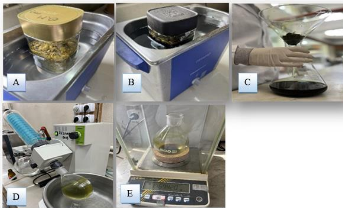
Figure 10. Photographs of the different stages of extract preparation from plant materials ( Matricaria chamomilla , Ocimum basilicum ). (A) Ultrasonication of MC; (B) ultrasonication of OB; (C) filtration of two plants; (D) Evaporation of MC; (E) Evaporation of OB.
