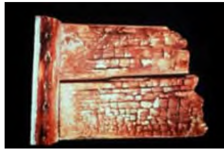
Figure 04: Image illustrant la pourriture brune ( http://www.alliancesudexpertise.com/insectes-a-larves-xylophages-parasites-du-bois.php )
