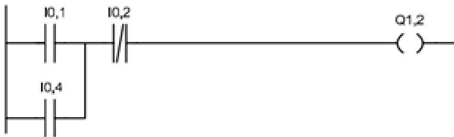
Figure 18. Example of a LD program
