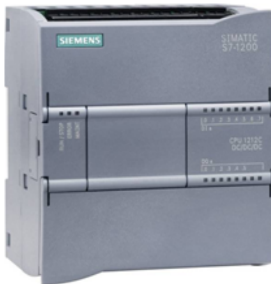
Figure 8. Example of programmable logic controller
