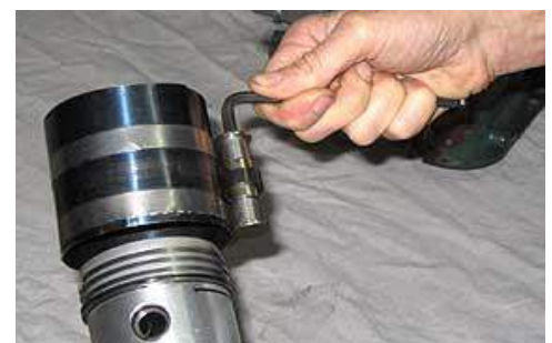
Fig.10a : Collier pou segments a piston
