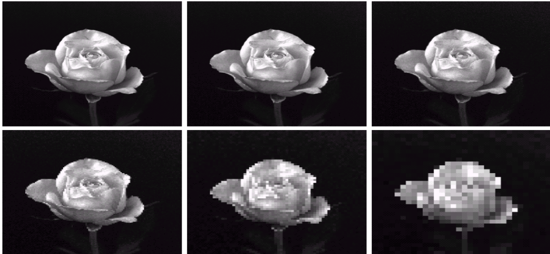
FIGURE 2.20 (a) 1024 \times 1024 , 8-bit image. (b) 512 \times 512 image resampled into 1024 \times 1024 pixels by row and column duplication. (c) through (f) 256 \times 256 , 128 \times 128 , 64 \times 64 , and 32 \times 32 images resampled into 1024 \times 1024 pixels.
